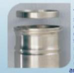
Scania diesels are clean. The unique Saver Ring, seated at top of the cylinder liner, removes all deposits from the piston top land on piston's upward stroke. Thereby permitting high and continuous load without any risk of coke built up lishing. The saver Ping and
