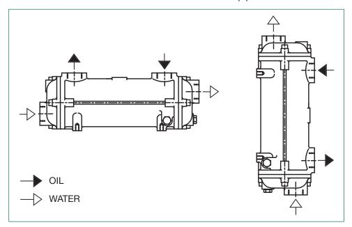
If the sea water supply is taken from the ship's main, ensure that the recommended flow rate cannot be exceeded. This will normally mean that an orifice plate must be fitted in the pipe work at least 1m before the cooler with the orifice size calculated to ensure that the maximum sea water flow rate cannot be exceeded. If these precautions are not taken, it is possible that the sea water flow rate through the cooler may be several times the recommended maximum which will lead to rapid failure.
